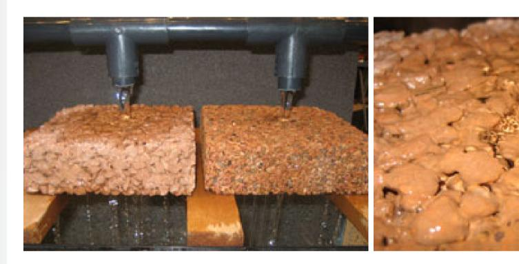
Water permeability experimental results 400cc Number of seconds when flowing down
